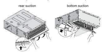
2 Clean the air filter. Use a vacuum cleaner or wash with water. If the air filter is very dirty, use a soft brush and neutral detergent.
